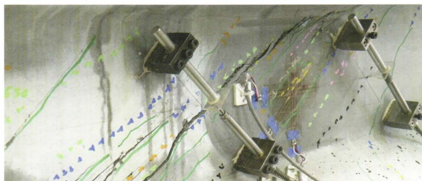
Pseudo-ductile, multi-cracking behaviour of a structure composed of an ultra-high performance fibre-reinforced concrete observed during a beam shear strain test conducted on the LCPC-Paris structural testing platform.
