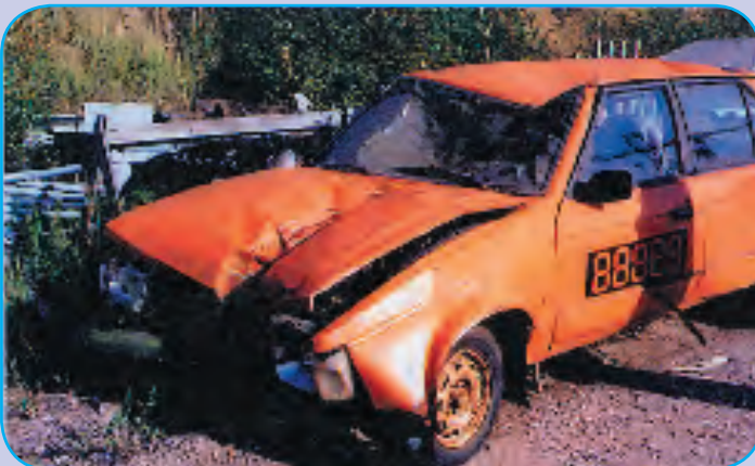
> Result of an impact test at 100 kph against an energy-absorbing lamp-post: the vehicle cabin is only slightly deformed – passengers wearing seatbelts would escape injury. (Sweden)
