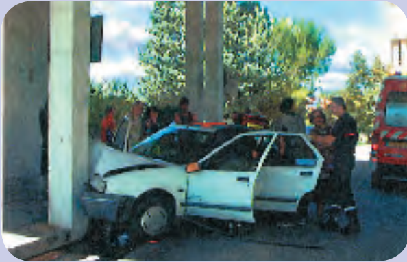
> Loss of control at low speed (40 kph) on a narrow street with poorly-parked cars. Impact against a pillar at an estimated speed of 20 kph; 1 person slightly injured. (Source: INRETS MA)
