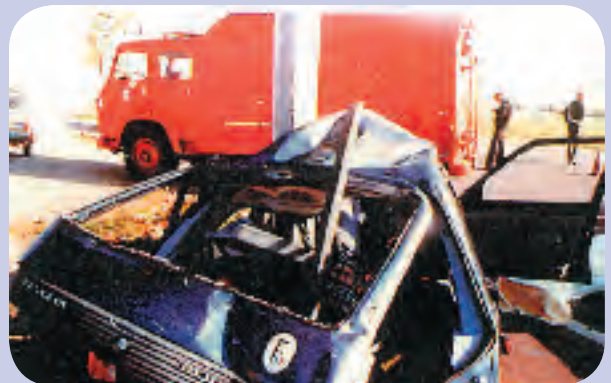
> Fatal accident in which a vehicle lost control and struck a lamppost. Side impact at an estimated speed of 40 kph.
