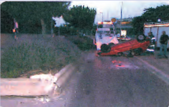
> Driver impeded at a junction, causing their vehicle to strike the kerb at 45 kph and roll over. (Source: INRETS MA)
