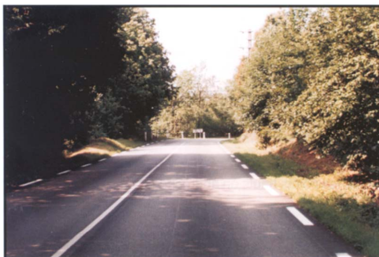
Approaching drivers cannot assess the length of the bend
