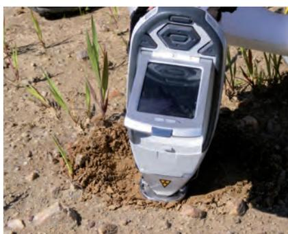
On-site measurement using an X-ray fluorescence spectrometer
