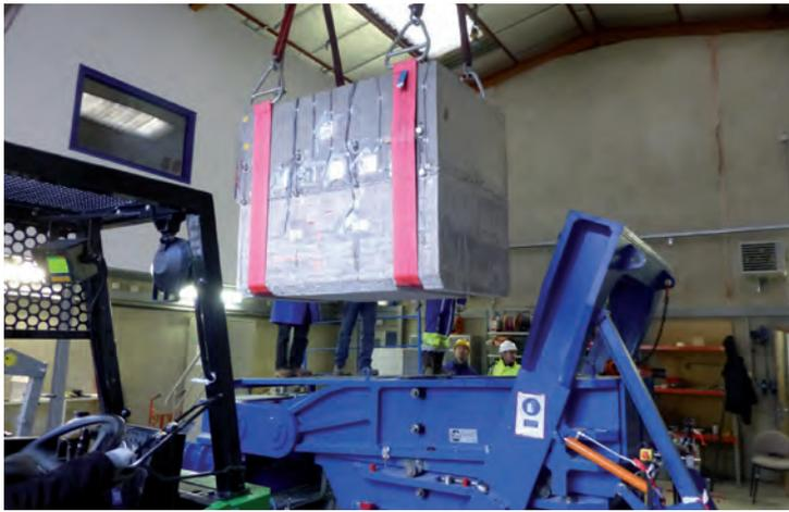
Setting up of a metric test-piece in Cerema's large-size direct shear unit
