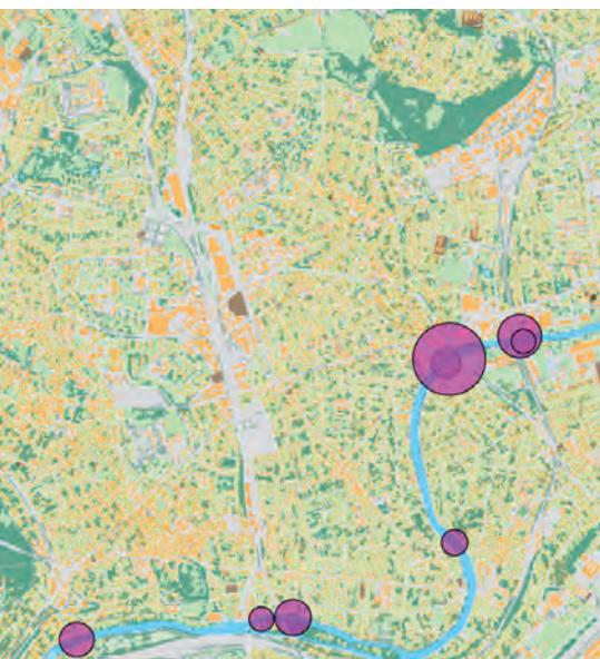
Example of mapping produced in the framework of the Trafipollu project on the relative distribution (fuchsia-coloured circles) of a pollutant (in this case copper) from automotive traffic, at the outlets of the studied rainwater networks flowing into the Marne river. It can be noted that the organization of the zone's sewage network tends to redistribute and concentrate the pollution, which is essentially emitted along the roadway at the center of this domain, upstream from the Marne
