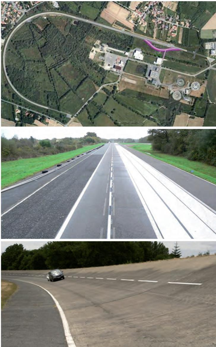
The ROSANNE (ROLLing resistance, Skid resistance, ANd Noise Emission measurement standards for road surfaces) European project aims to define common practices shared across Europe in terms of measurements of road usage properties such as grip, or skid resistance, noise and rolling resistance. This pre-standardization project (2013-2016) made it possible inter alia to conduct several skid and rolling resistance measurement campaigns of IFSTTAR's test track surface in Nantes.
