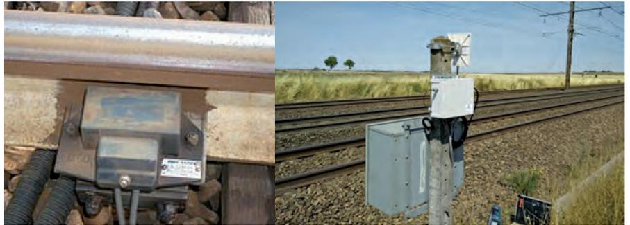
Instrumentation of two axle counters on the Paris-Orléans railway line using IFSTTAR technological bricks and algorithms
