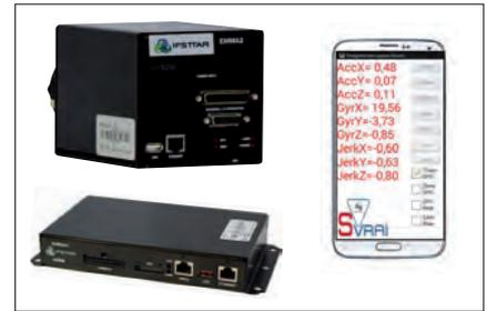
Emma units (In-vehicle accident mechanisms recording units): version 2, version 3 and “EmmaPhone” version
